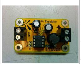
This is a step-down DC-DC converter based upon the LM2574 IC.
