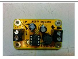
Carefully insert the 8 pin LM2574 IC.
