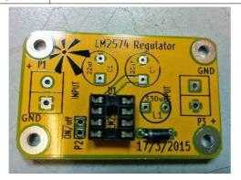
Check the orientation of the diode. The silver line should line up with the arrow mark on the PCB silkscreen.
