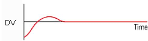
Figure 8: Proportional plus Integral plus Derivative Control (Adapted from [14])
