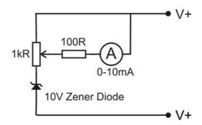
The basic idea is to drop some voltage across a zener diode. An ammeter is used to read the voltage by using a resistor (remember Ohms Law? V=IR). The lowest voltage that can be read will be equal to the rating of the zener diode (in this case 10V). The scale can then be chosen through the use of the correct resistor values and some calculation (see below). The variable resistor allows fine tuning of the scale, especially when the exact resistor values are unobtainable.
