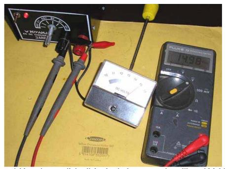
Adjust variable resistor until the dial value is the same as the calibrated Multimeter. Check the scale by running through the range of voltages.
