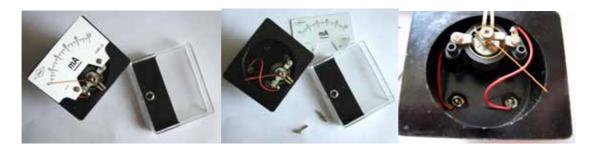
Drill a hole large enough for the variable resistor to turn. Glue the strip board in place so that the variable resistor is accessible, with a screwdriver, through the hole:
