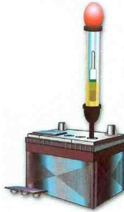
Specific gravity is measured using a *hydrometer*. This device uses a small floating weight which shows the density of the electrolyte. The reading is affected by temperature. Follow the hydrometer instructions for correct reading. **Always wear gloves and goggles.**
