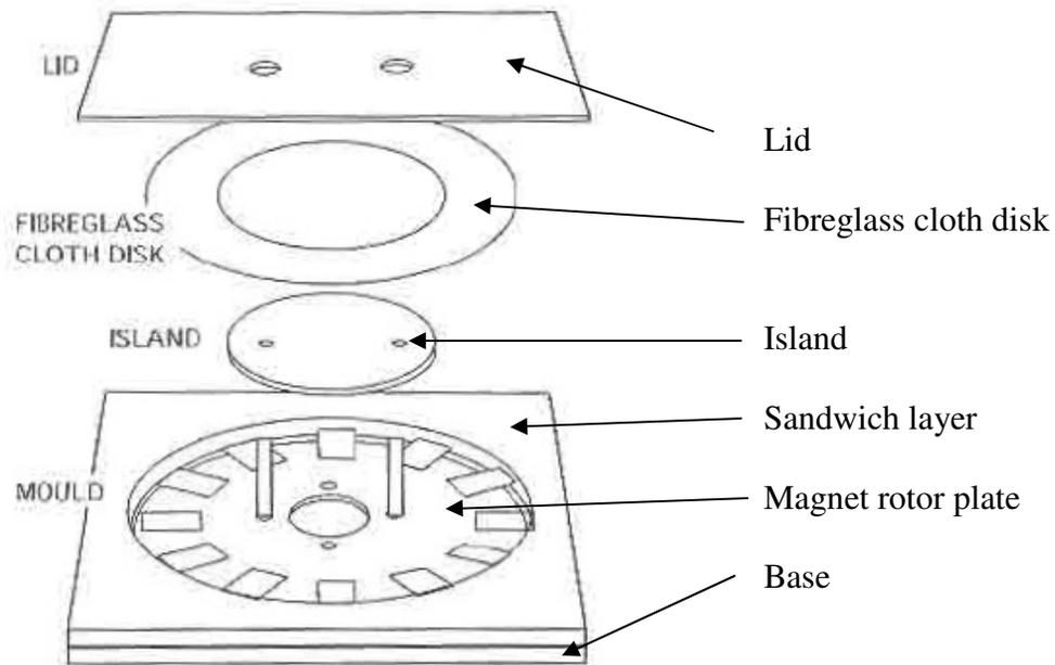
SIBAT have fabricated aluminium rotor moulds for the casting of the rotor disks (see CAD drawings/Rotor mould). The mould consists of a base, sandwich layer, island and lid. 2 sets of moulds are available so the magnet rotor plates can be cast at the same time. Ensure the moulds are clean and smooth, and all the necessary bolts, nuts and washers are available. The rotor disks should be cast on a flat surface in a well ventilated area. Allow 2-3 hours for this task with a minimum of 2 people.
