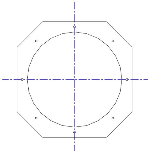
First cut out the 2 fibreglass cloth disks, 360mm diameter with a 210mm central hole.
