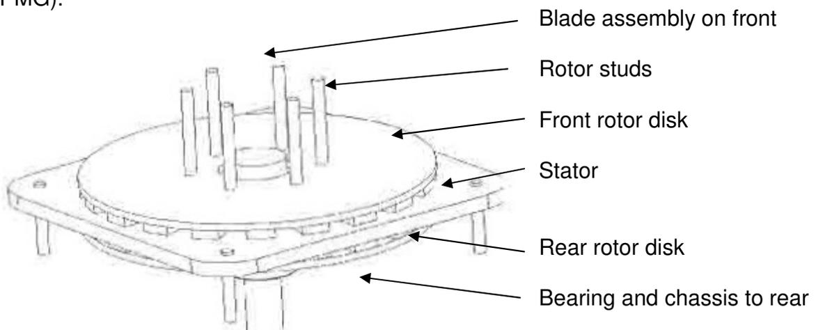
The rotor disks are connected to the bearing on the chassis by 6 rotor studs. The blade assembly is attached to the rotor studs on the front side. 2 rotor studs pass through each blade root.
