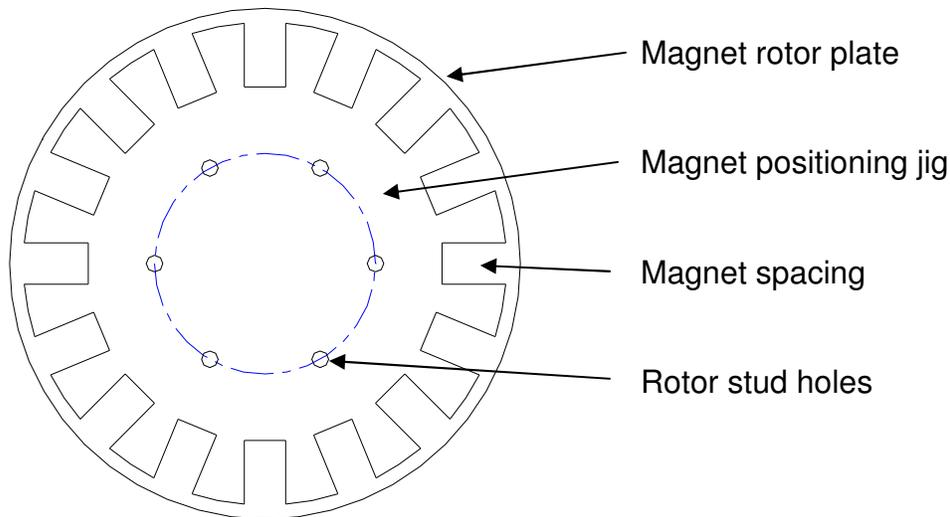
The first step is to sand or grind any mill-scale off the area where the magnets will sit, and clean them to remove any grease. Then position the magnet positioning jig on one of the magnet rotor plates. Since there is only one magnet positioning jig the 2 magnet rotor plates will be done separately.
