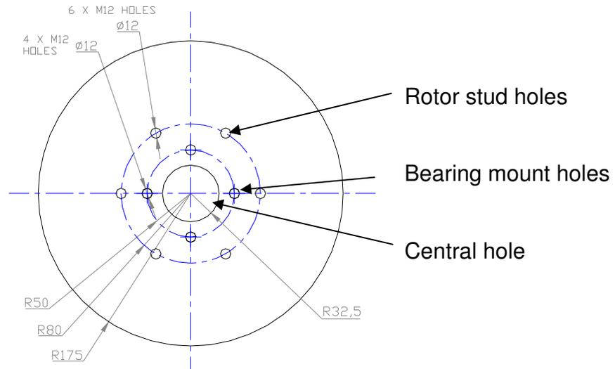
The large central hole is to allow the rear magnet plate to sit flat on the bearing flange - it is also useful to have it on the front magnet plate. The hole can be made with a holesaw (or a laser if available). If the cost of making the central hole is very high it is possible to manage without the hole. Instead of the rear rotor plate being tight against the bearing flange it would have to be separated by 2-3 nuts on the bolts to avoid the bearing cap interference.
