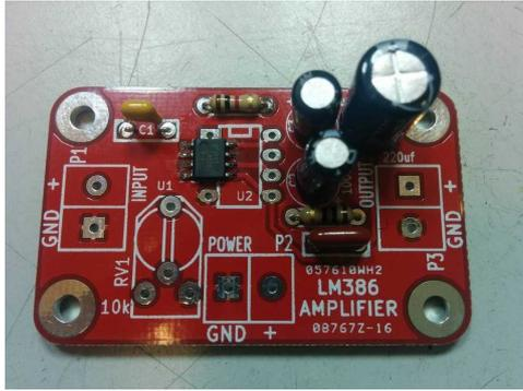
Capacitors C1 and C4 can be installed in either direction.
