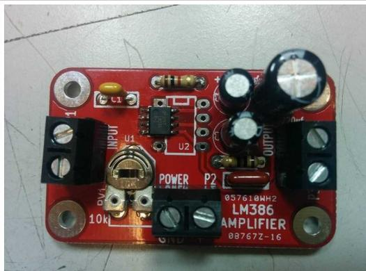
There are three 2-way terminal blocks. These have the connections pointing away from the PCB, as we need to be able to connect wires in to them.
